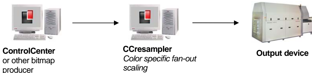
Example of configuration for fan-out compensation using Ccresampler as anamorphic scaling engine
