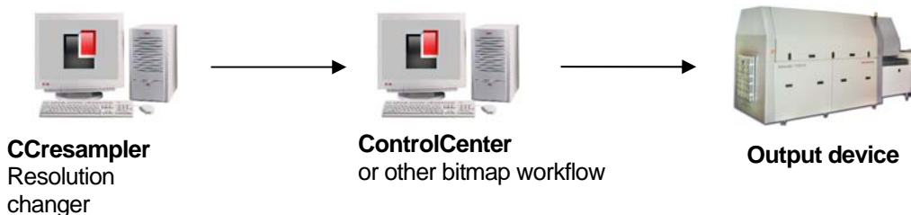
Example of configuration for normalizing resolution of incoming bitmaps. CCresampler is capable of changing resolution up or down.
